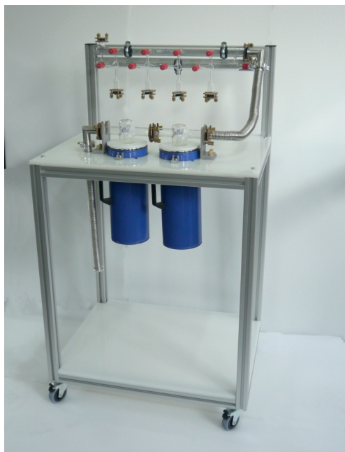
Pump stand with Schlenkline, glass cooling traps and detachable Dewar flasks
