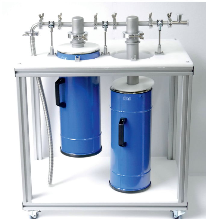
Pump stand with large metal cooling traps and detachable large Dewar flasks
